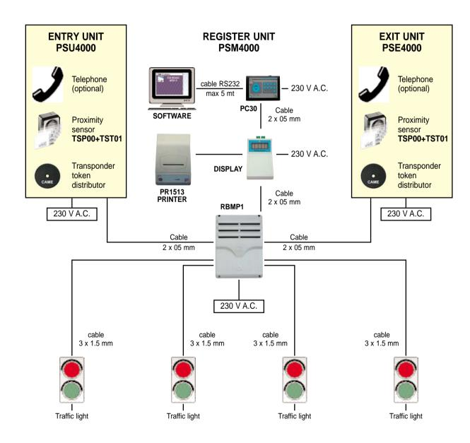
N.B. The entry and exit automation systems (automatic barriers or other) are directly controlled by their respective units and it is also possible to effect control from a PC. The PSM4000 register unit is exclusively for use with the RBMP1 - PC30 and RBPARK software.
