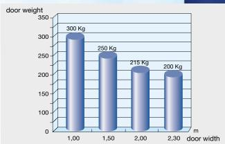
FAST can be applied to single doors up to 2,3 mt (7,5 ft) wide, with distances of up to 200 mm (8") between the hinge of the gate and the edge of the column.
