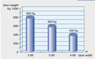
FERNI can be applied to single doors up to 4 mt (12 ft) wide, with distances of up to 380 mm (15") between the hinge of the gate and the edge of the column.
